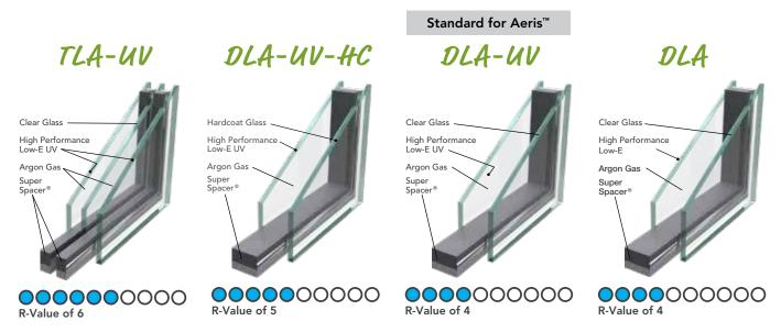
Several other double and triple glazed glass packages are available, including with Krypton Gas (triple glazed only) as well as Hard Coat and Low-E options.
